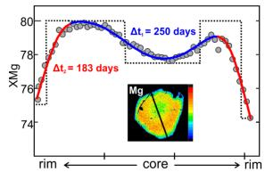
**Fig. 2** depicts a typical result of stepwise modelling of a zoned crystal. Dots: Analytical data; Black dashed line: Initial profile; Black line: Best fit diffusion model. Inset: Mg distribution map (the darker the colour the higher the Mg concentration); Black arrow indicates the direction of the microanalytical traverse. Sequential modelling reveals two timescales ( $\Delta$ t1,  $\Delta$ t2) corresponding to the residence of the crystal in two different magmatic reservoirs.
